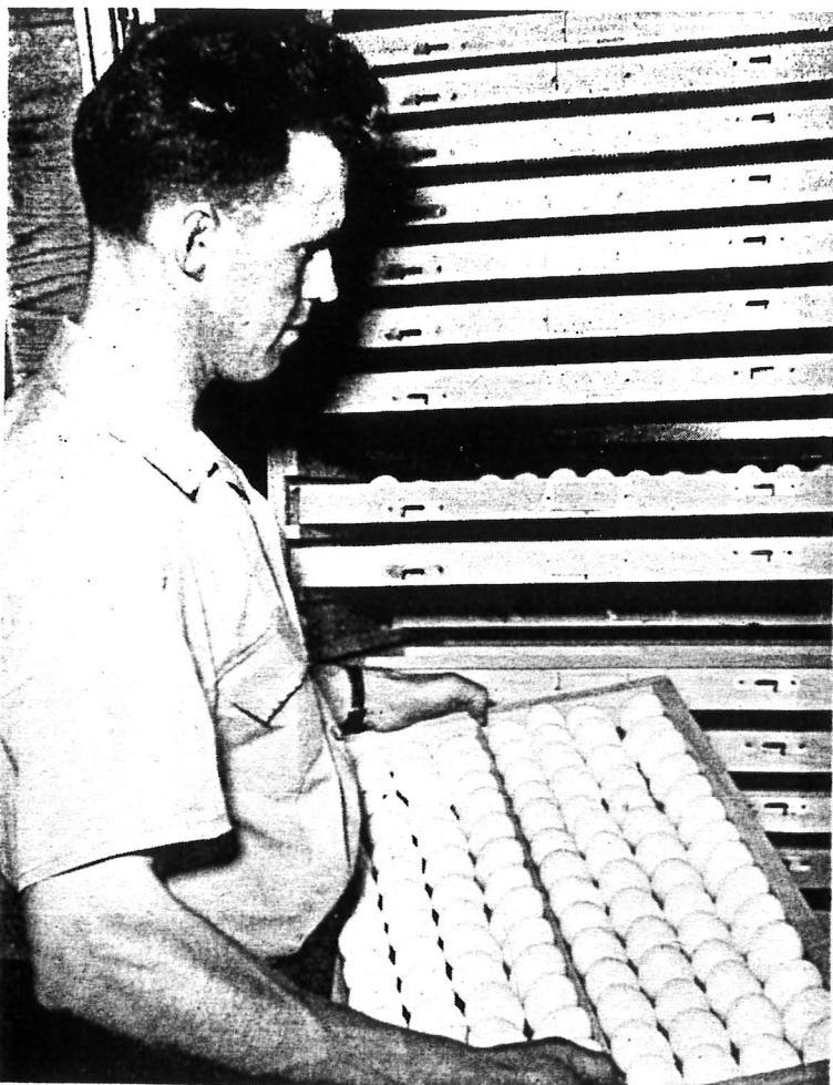
Into the incubator go these trays of eggs. Dryden Fleenor is placing them in the racks. Chicks are hatched scientifically through precision control of temperature, ventilation, and humidity. This machine has a capacity of 12,000 eggs and is so designed that temperature is controlled to within one-fifth of a degree.
